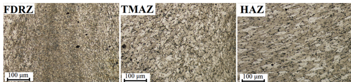
Fig. 9. Optical microstructure of the AA2024 weld joint.
