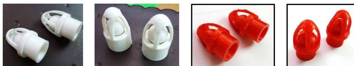
Fig. 6. The 3D printing of an artificial conical caged ball heart valves.
